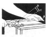
If strap needs further tightening, pull long handle back from position "A" to position "B". Tighten strap with short easy strokes from "B" to "C".
