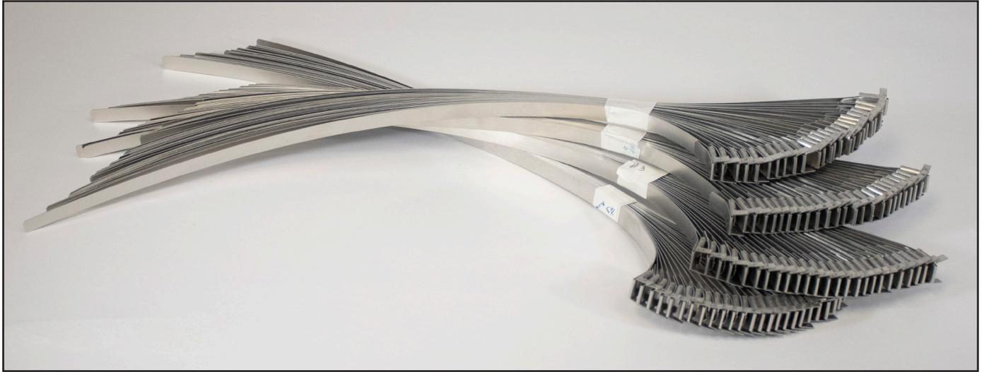
Fabstraps are customized fabricated strapping with wing seals attached using aluminum or stainless steel. The strapping is of specific lengths as required, and is supplied in ready to use units. They are used to secure field applied metal jacketing and/or insulation in place.
